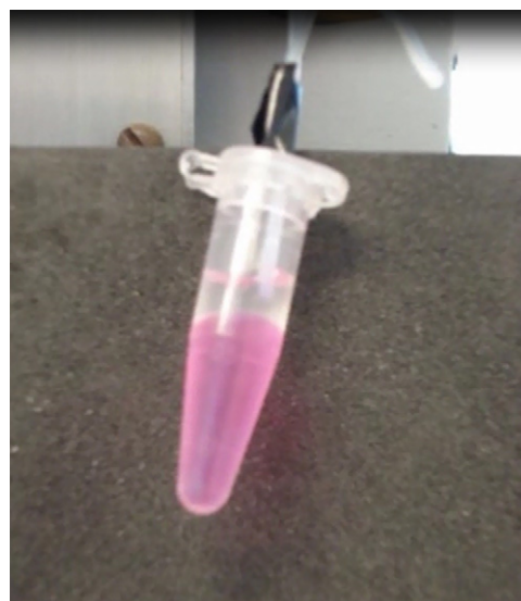
Fig. 2. Extraction procedure of blank solution measurement. The slight color of the upper organic phase is caused by low amount of extracted AP. (For interpretation of the references to color in this figure legend, the reader is referred to the web version of the article.)
